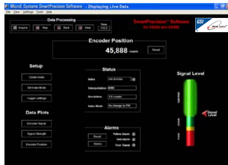
Setup and Status screen when used with Mercury 3500Si and 3000Si encoders
