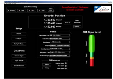
Setup and Status screen when used with Mercury 3000SiDAA and 3000DAA encoders
